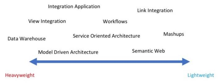
Schema of the different data integration strategies placed according to their level of integration. From left to right we go from heavyweight to lightweight integration level.
