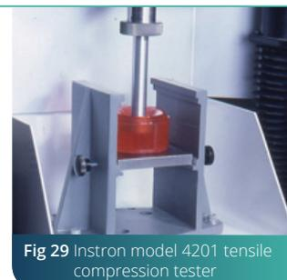
Fig 29 Instron model 4201 tensile compression tester
