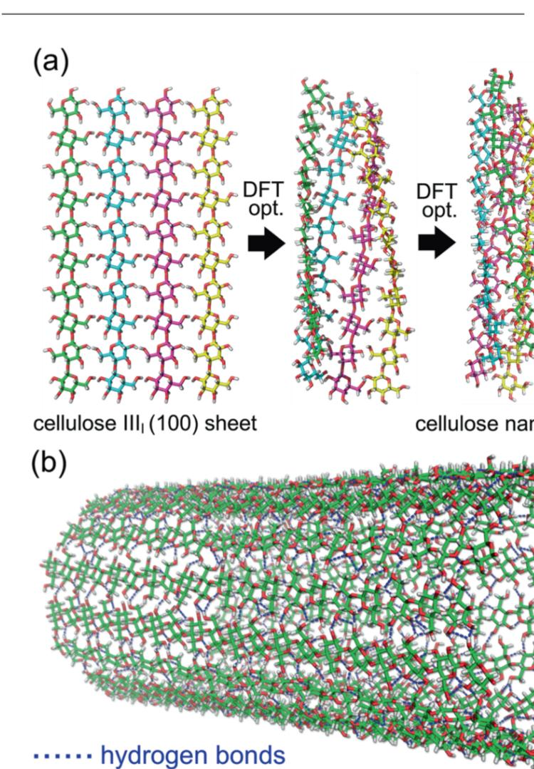
**Figure** : Formation of cellulose nanotubes (CelNTs) from cellulose IIII (100) sheets, as predicted by the DFT calculations. b Average structure of the CelNT model in benzene evaluated by MD calculations
