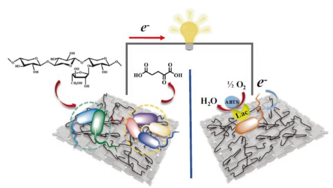
Schematic drawing of electron transfer route and catalytic reactions in the proposed two-compartment xylan/O2 MFC. The system was composed of the enzyme-engineered bacterial consortia-based bioanode and E. coli-Lac-based biocathode
