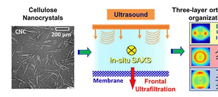
For the first time, a typical three-layer orthotropic structure that resembles the articular cartilage organization was achieved in one step during the FU/US process. The result comprises a first layer composed of CNCs having their director aligned parallel to the horizontal membrane surface, a second intermediate isotropic layer, and a third layer of CNCs with their director vertically oriented along the direction of US wave propagation direction.
